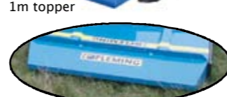
Closed in safety guard built into frame.
