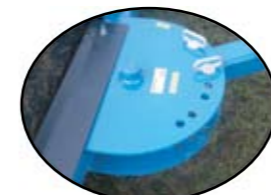
Lead roller can be set for use with either 2.5m or 3m following roller
