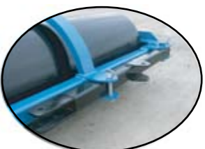
Lead roller drawing arm can be folded for drawing rollers in-line for easy field access
