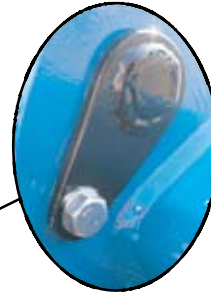
Locked pivot pins to prevent excessive wear
